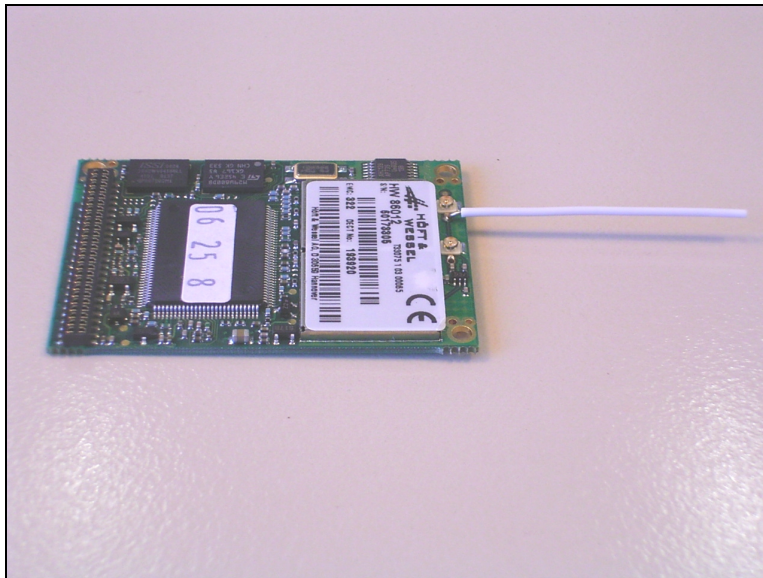
Figure 9: HW 86012 standard version with wire antenna mounted on ANT1 port.
