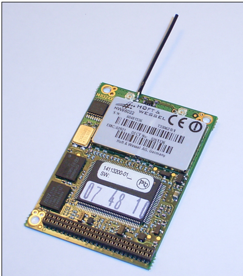
Figure 10: HW 86022 standard version with wire antenna mounted on ANT1 port.
